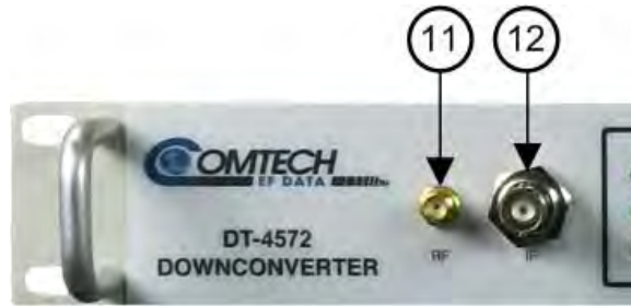
Figure 4-14. Front Panel Sample Test Point Connections
