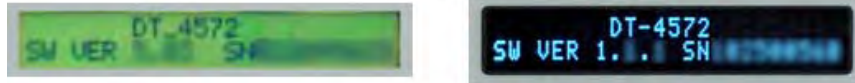
(LEFT) Liquid Crystal Display (LCD) – Initially Released Chassis (RIGHT) Vacuum Fluorescent Display (VFD) – Current Production Unit
